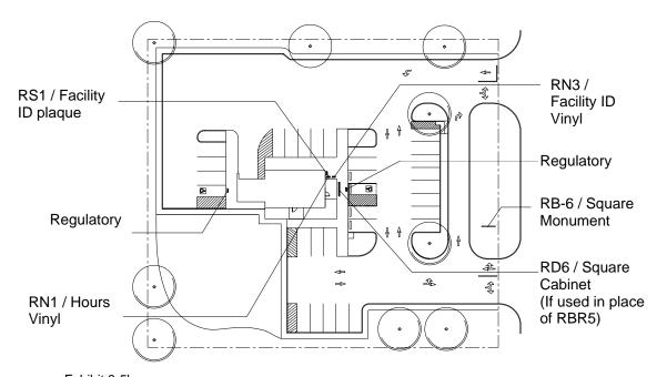
Exhibit 3-5b Typical site plan showing sign placement for SSBD plan 15
