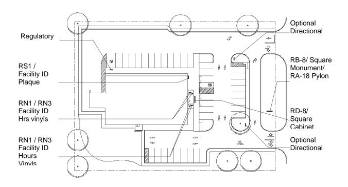
Exhibit 3-5k Typical site plan showing sign placement for SSBD plans 40, 50, 65A, 80A, and 100A  $\,$
