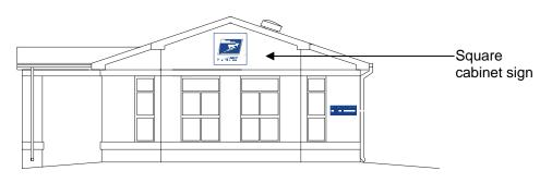
Exhibit 3-5c Typical elevation showing placement of Square Cabinet sign (if provided) and Facility / Station ID Plaque for SSBD plan 15
