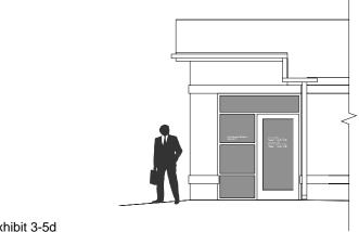
Typical elevation of entrance with vinyl placement for SSBD plan 15
