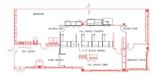
\*Note, the graphic above is for visual reference and to show adjacencies only. See paragraph below for clarification on the requirements to accommodate the 3'-0" opening between the counters.
