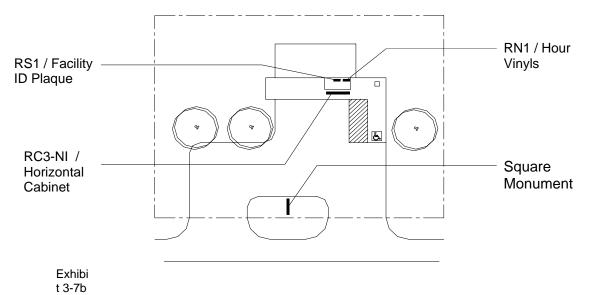
Typical site plan of Modular Building with sign placement
